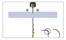
Route the coaxial cables through the hole in the panel. Align the antenna properly and press down to secure the adhesive base in place. Note: Avoid sharp bends when routing coaxial cable.
