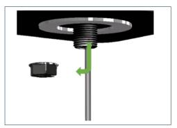
Unscrew the split steel nut from the antenna body and slide the the coaxial cable out through nut and washer.
