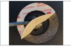
Ensure the mouting surface is clean and all debris, dust, or any other contaminant is removed. Remove the protective liner from the pre-installed base adhesive on the antenna.
