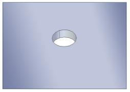
Determine where the antenna is to be mounted, please ensure this is a flat surface. Drill a 16mm [5/8"] diameter hole.
