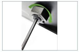
Insert the coaxial cables through the washer and steel nut and slide them upwards. Tighten to secure the antenna in place. Ensure the nut is fully tightened.
