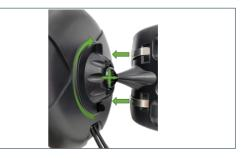
Insert the ball joint firmly into the socket on the back of the antenna body and slide the tightening nut into the antenna housing's back plate to secure in place. Adjust to the desired antenna orientation on the bal joint and tighten the nut to fix the antenna in place.
