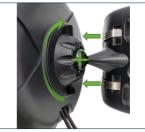
Insert the ball joint firmly into the socket on the back of the antenna body and slide the tightening nut into the antenna housing's back plate to secure in place. Adjust to the desired antenna orientation on the bal joint and tighten the nut to fix the antenna in place.
