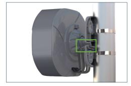
Optional: Route cables through the cable guide on the mounting plate
