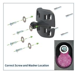
Using the mounting plate as a guide mark the position of the screws to the desired location. Drill holes for wall mount studs(6mm[1/4"] diamter, min 25mm[1"] depth) and secure the studs in place. Position the washers into the mounting plate, insert the screws through and into the wall studs. Drive the screws in and tighten to secure the mounting plate in place
