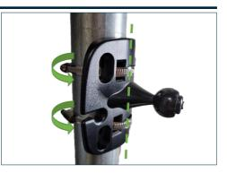
Loop the mouting straps around the pole at the desired position and tighten the strap until the mounting plate is fixed. Use the self centering feature to guide the mounting plate onto the pole
