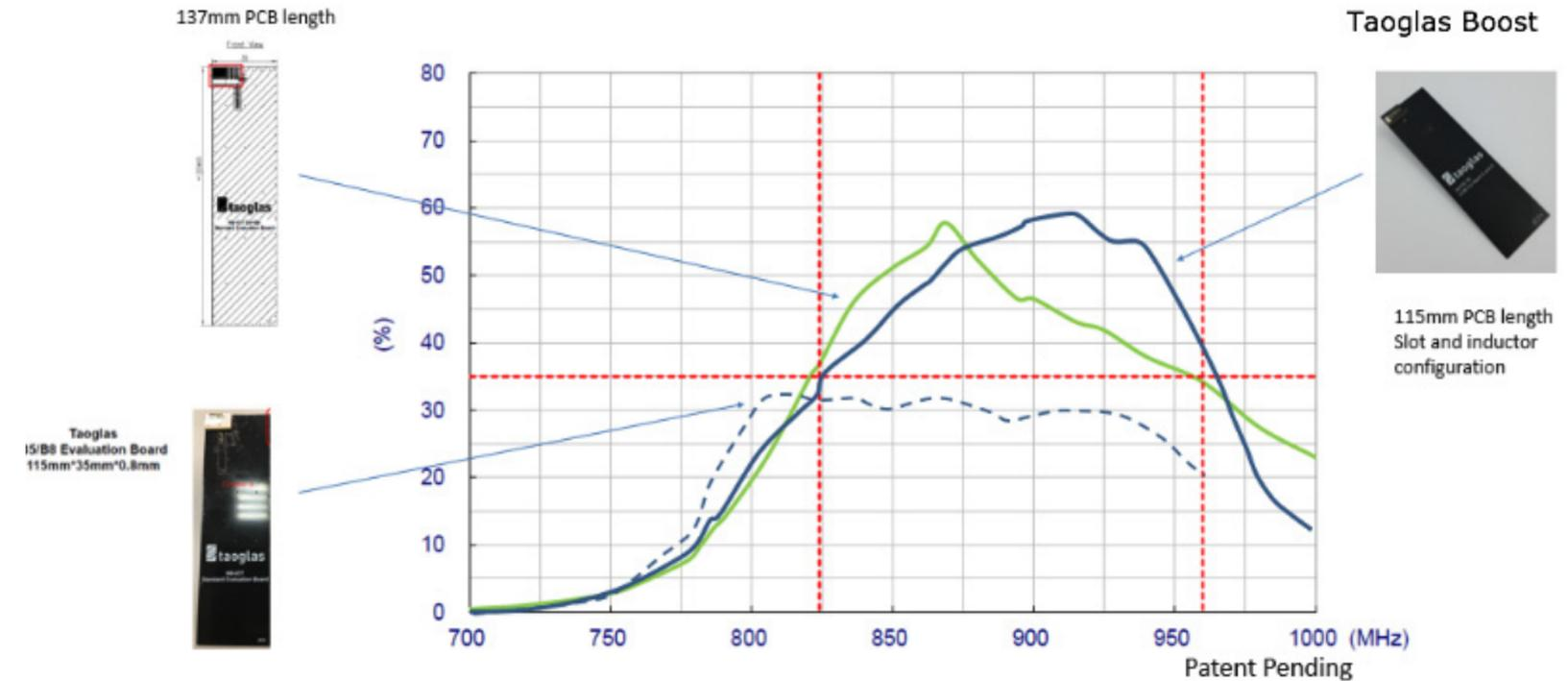
Fig 7. Comparison of efficiency performance for Taoglas Boost enabled ground plane and ground planes without Taoglas Boost modification
