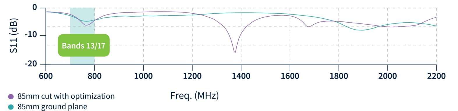
Fig 5. Efficiency and Return Loss with and without optimization applied to PA.710 evaluation board
