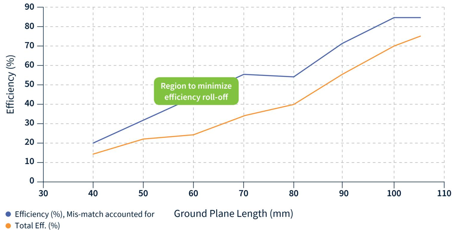
Fig 2. PA.710 Total efficiency and potential efficiency improvement when accounting for mis-match loss
