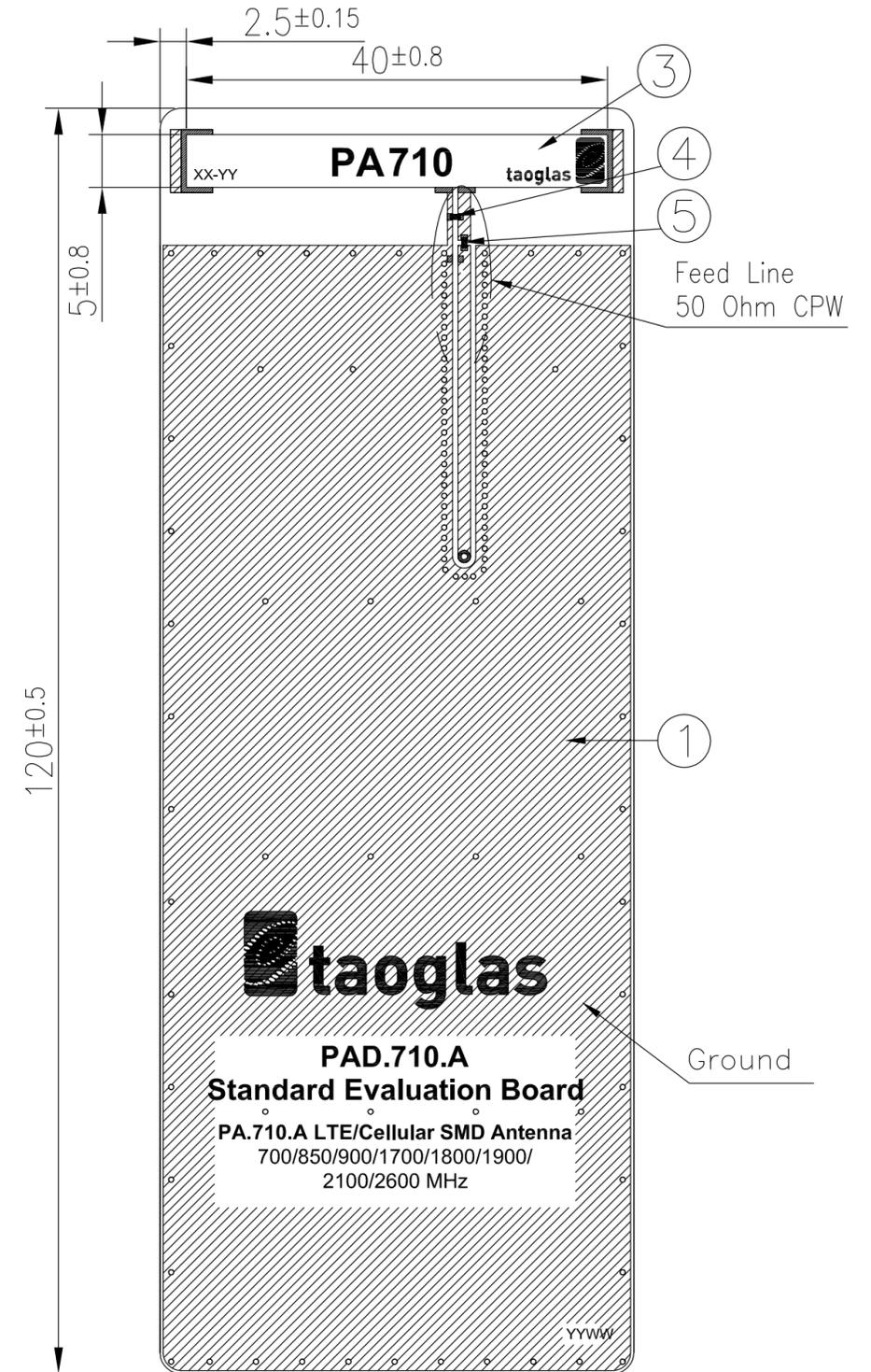
Fig 1. Cut-down test for PA.710, where the ground plane dimension is reduced and performance is tracked
