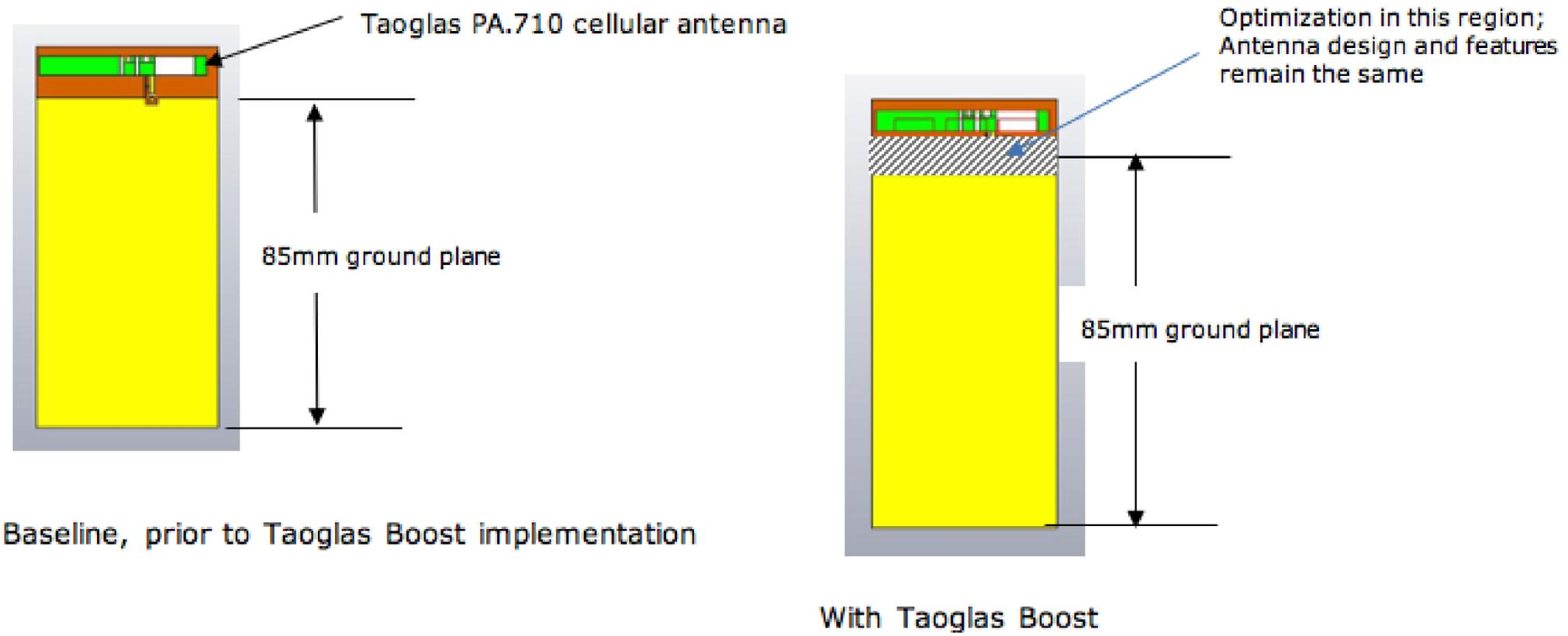
Fig 6. PA.710 antenna and evaluation board reduced in length to 85mm
