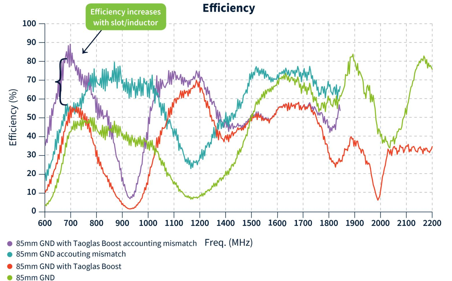
Fig 3. PA.710 with ground plane reduced from 106.5mm to 85mm
