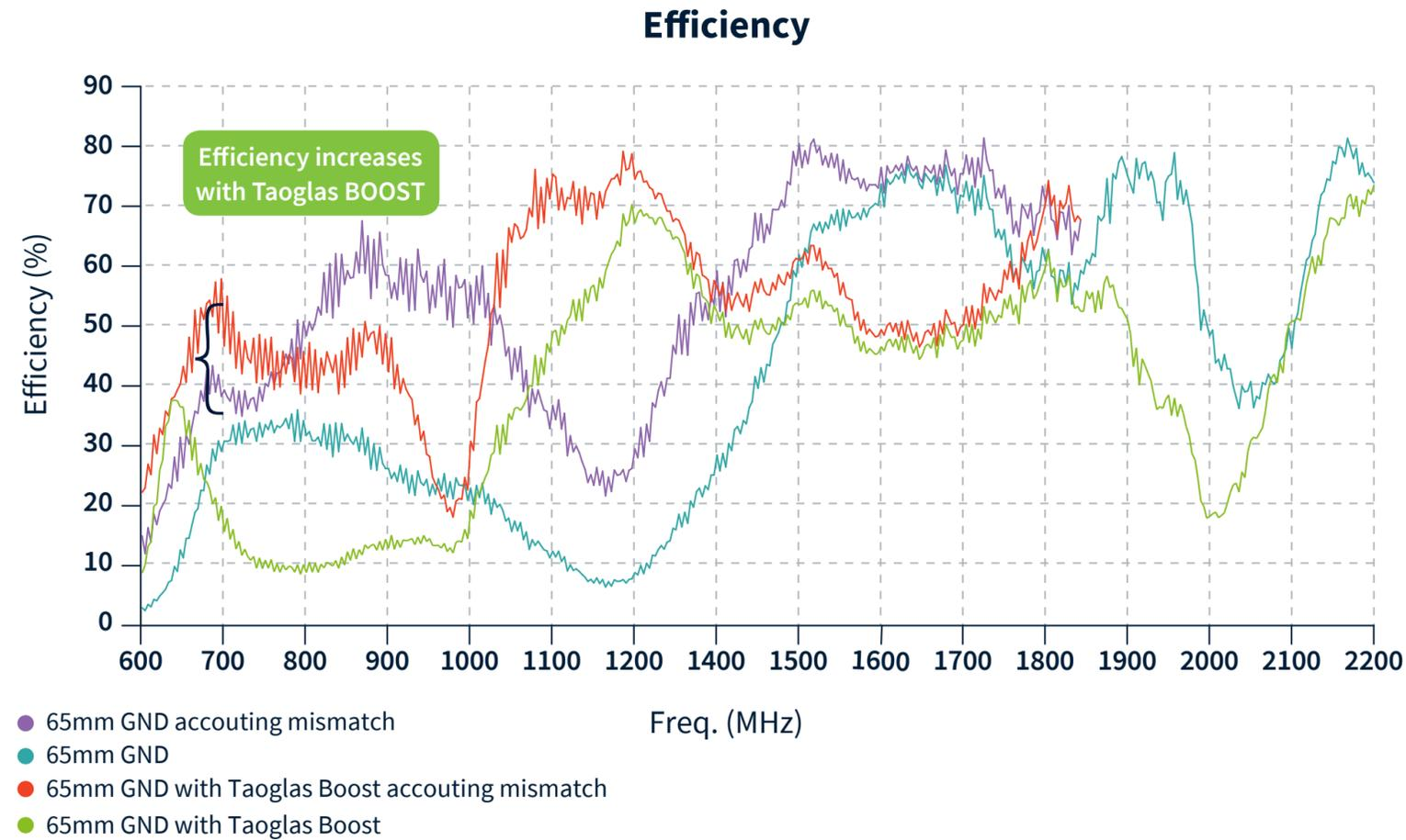
Fig 4. PA.710 with ground plane reduced from 106.5mm to 65mm
