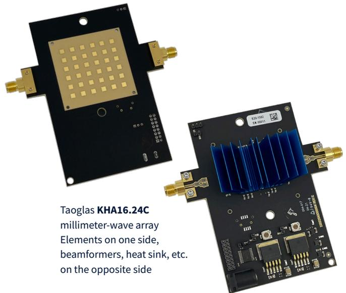
Taoglas **KHA16.24C** millimeter-wave array Elements on one side, beamformers, heat sink, etc. on the opposite side
